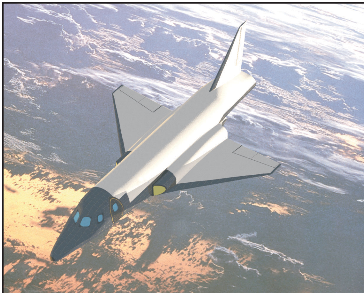
A conceptual illustration of the Rocketplane XP, a 4-seat fighter-sized reusable suborbital aircraft.
