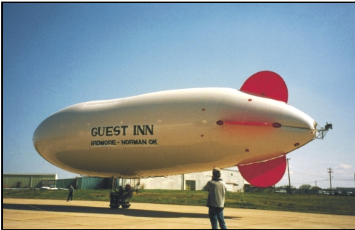
Marvin Polzien's second blimp design, ready for flight. Note gimbaled pitch/yaw engine on tail.
