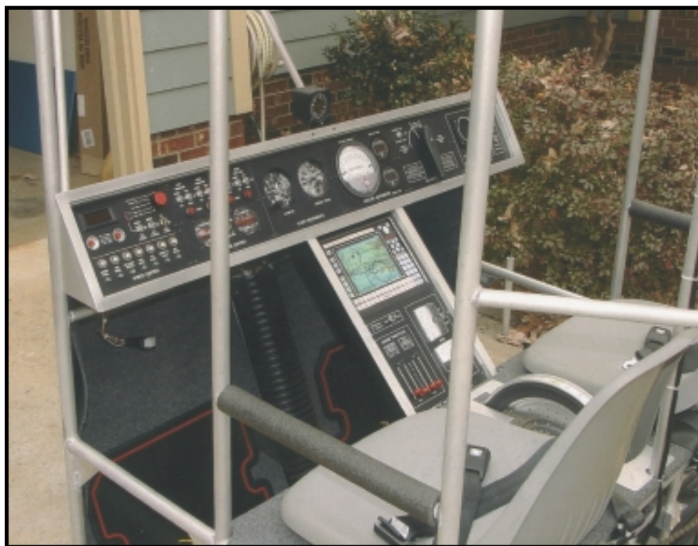
The pilot and passenger compartment of the blimp car. Instruments include compass, altimeter, rate of climb, water pressure gauge, outside air temperature, and temperature inside the envelope. On the right side of the panel is valve handle for controlling pressure in the ballonets. In the center console is a bit of whimsy: a picture of a fancy GPS/MFD unit-- maybe later!
