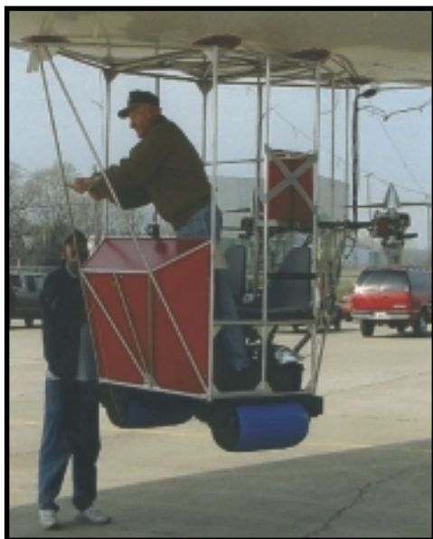
Ready for takeoff! Note that the main engines are rotated vertical to produce upward thrust.
