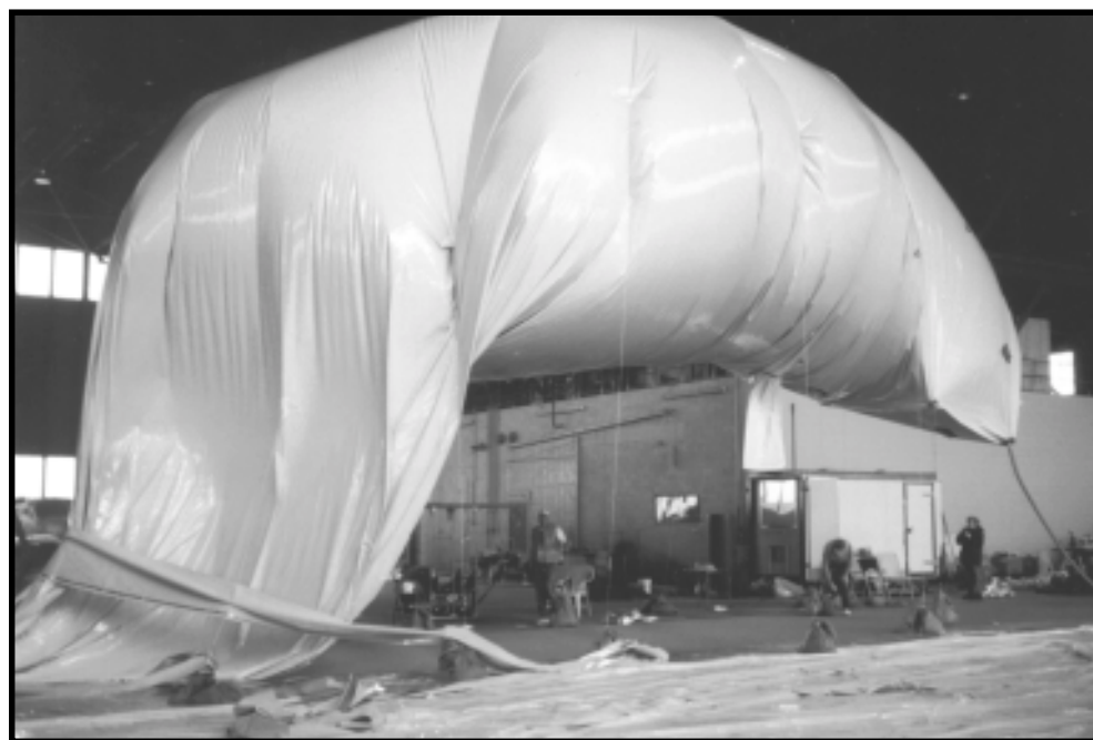
Looking like some gigantic man-eating bug from a B-movie, the blimp is being filled with helium. This filling was with the improved procedure, starting from the rear and working forward-- a sandbag is visible at the left side of the photo.
