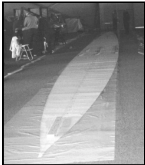
The gore pattern laid out for cutting. The Oklahoma Aviator, January 2003, Page 8
