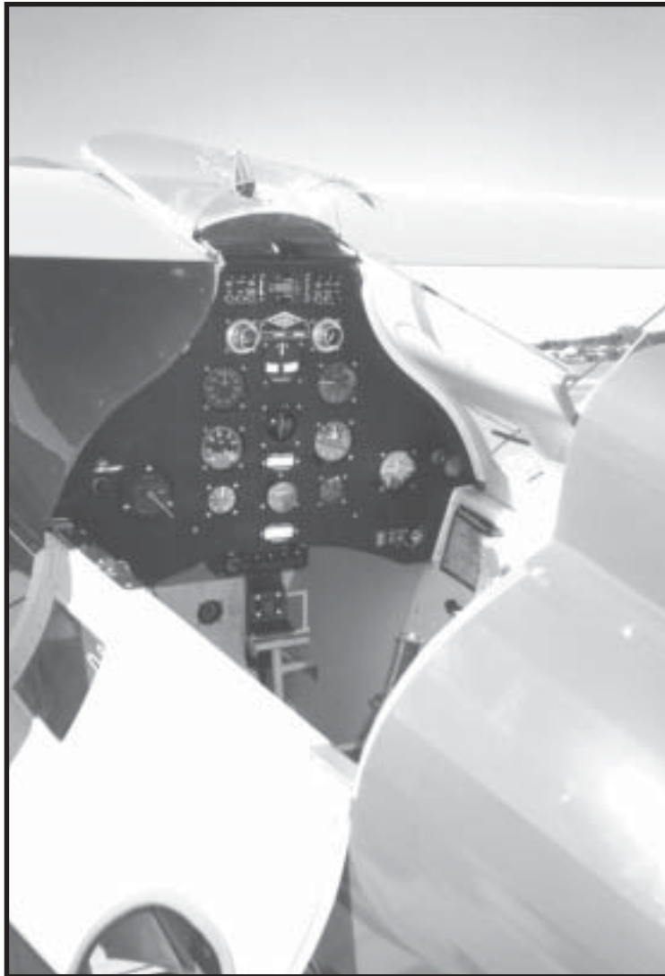
The Super Solution cockpit. The 3'-high "canopy" slides back and the sides are raised in position. Stop and consider the view of the world outside from the pilots position!!
