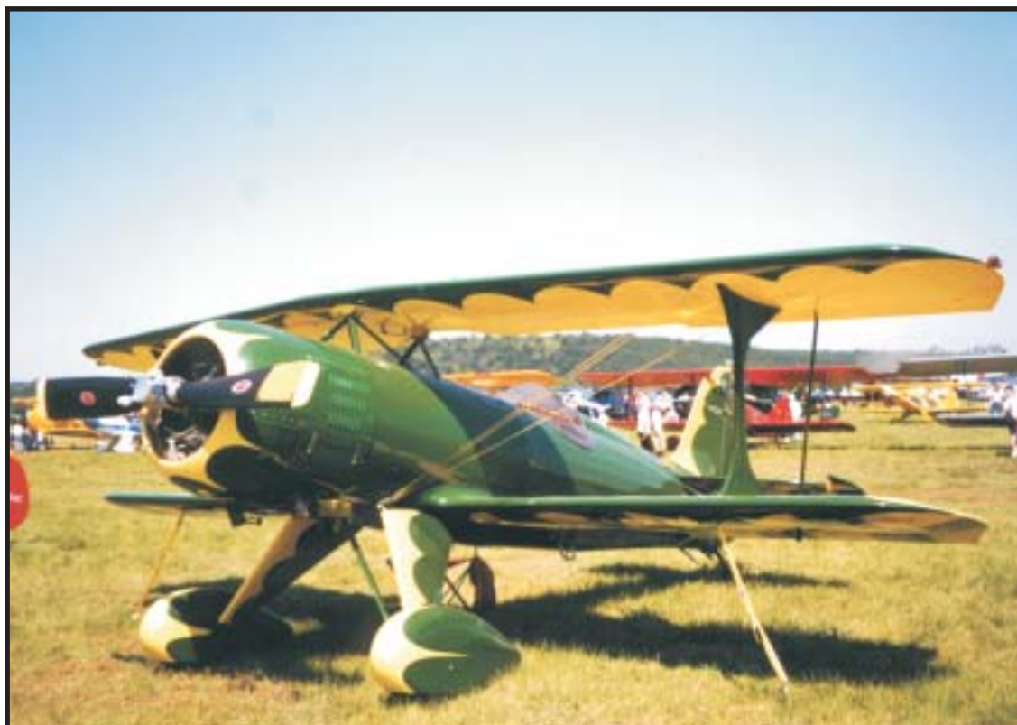
Blue skies, green grass, and cool weather surround this beautiful Culp Special, a modified Steen Skybolt design with a Russian 300-hp M-14P "round motor."
