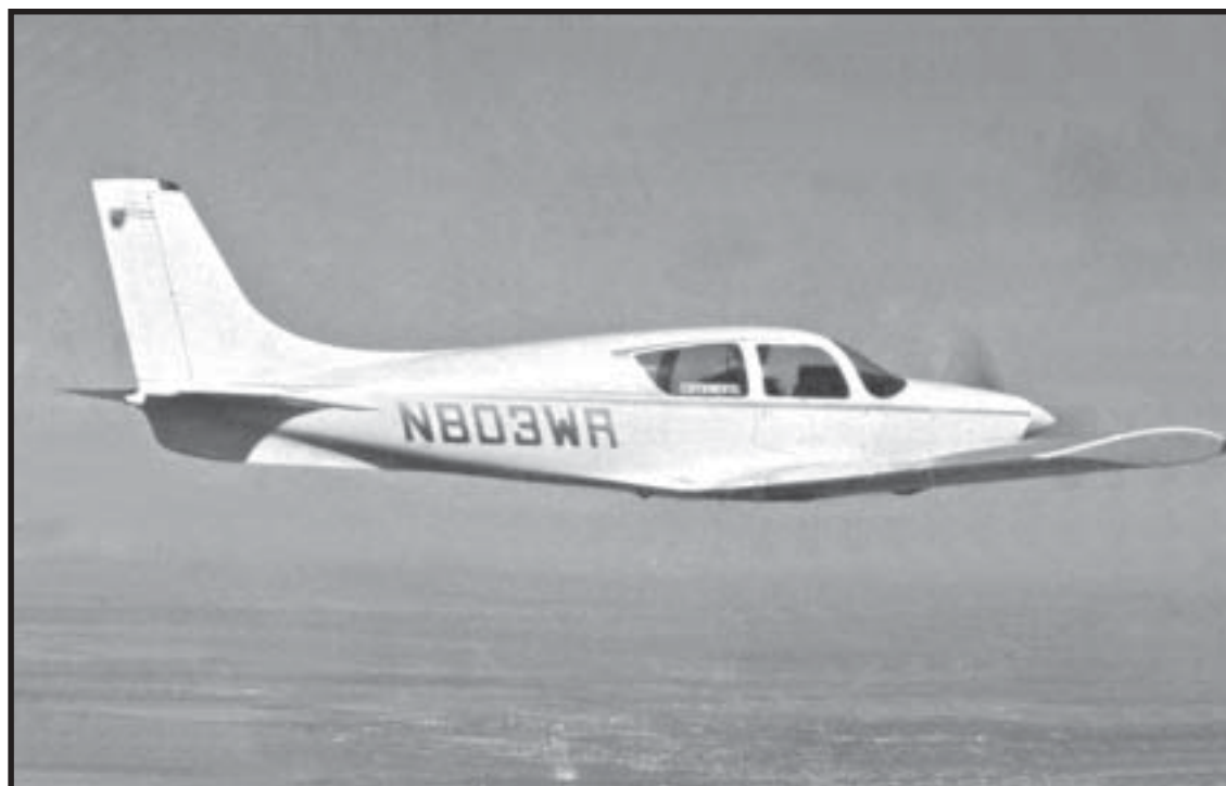
The second Windecker Eagle certification prototype, N803WR. Note the added ventral fin below the horizontal stabilizer, one of the changes made to eliminate the flat spin problem encountered by the first prototype, N802W.
