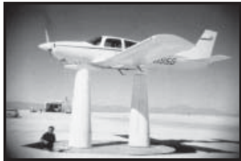
Windecker Eagle N4195G mounted on the RATSACAT pedestal in New Mexico, undergoing the beginnings of stealth testing
