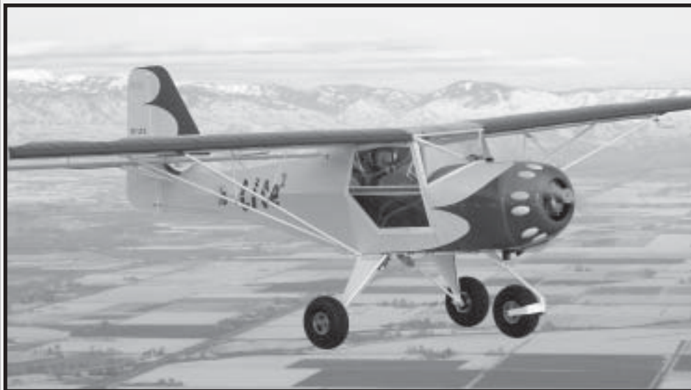
The Kitfox Lite Squared, a big-tire, big-engine, two-place version of the Lite.
