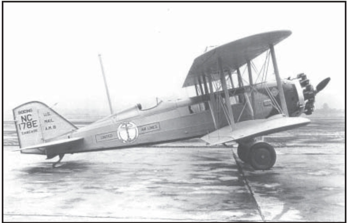
The Boeing Model 40-B-4, the very latest airliner technology when introduced in 1940. The pilot occupied the rear cockpit, while four passengers were comfortably seated inside the cabin. Note the United Air Lines logo on the side of the fuselage. Also note the enormous seat pitch: a seatback is visible at the rear of each cabin window! Today's airlines should definitely take a clue from the past!
