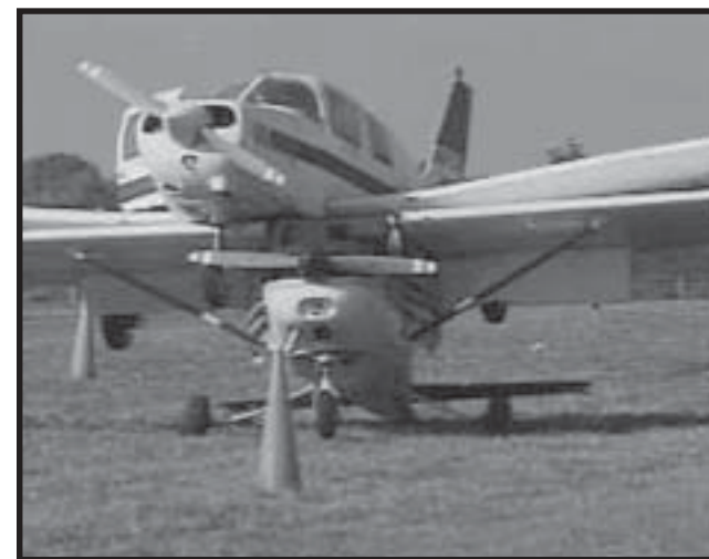
Piper PA-28 Cadet locked together with Cessna 152 after a midair collision and a safe landing at the Plant City Municipal Airport, Plant City, FL.
