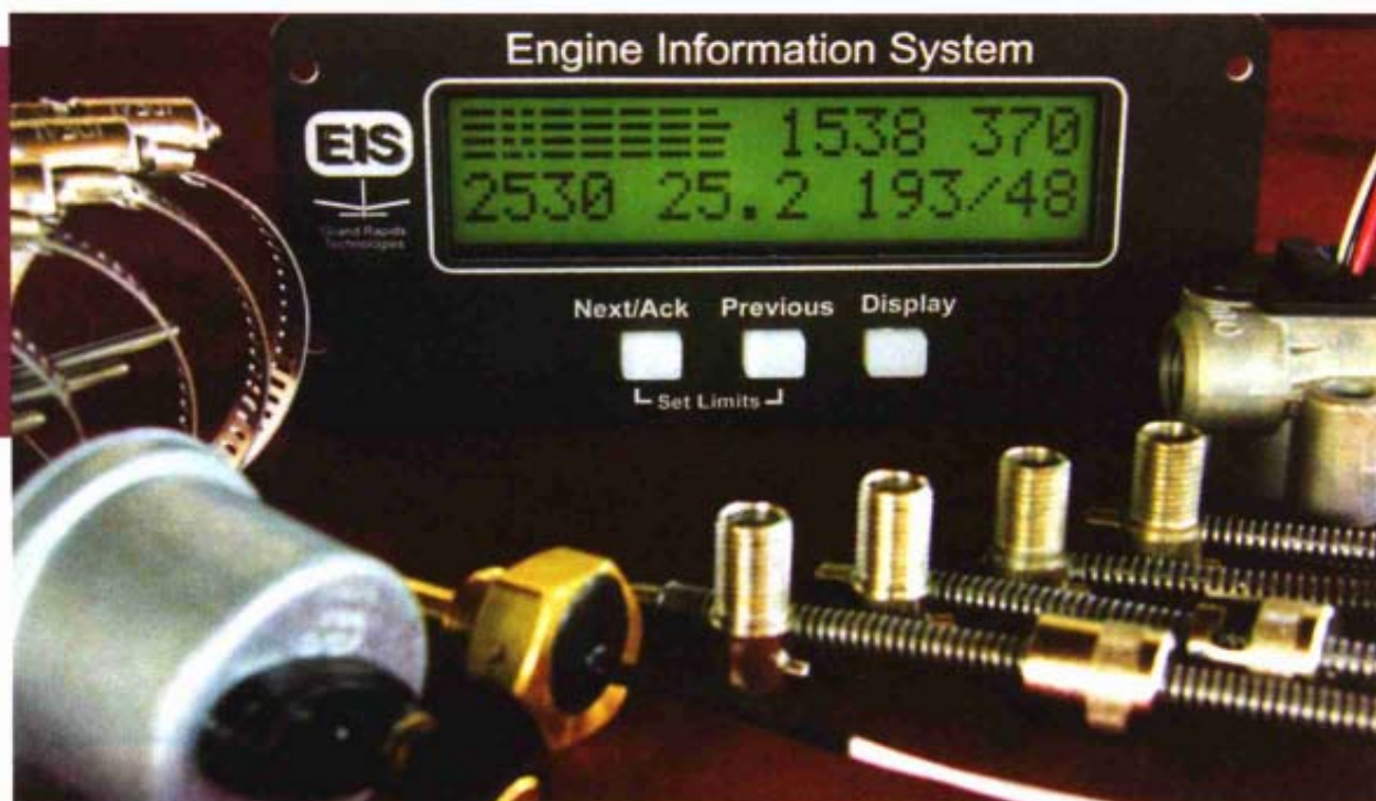
A typical engine information system (EIS) and some of its transducers.
